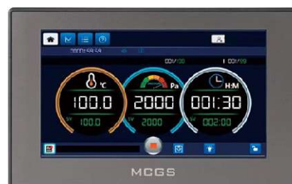
Touch Screen HMI Display for Vacuum and Temperature control with 3 level password protected user management for FDA requirement, Data storage, PC and Printer Connection facility
